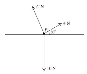
A particle P has weight 10 N and is in limiting equilibrium on a rough horizontal table. The forces shown in the diagram represent the weight of P, an applied force of magnitude 4 N acting on P in a direction at 30° above the horizontal, and the contact force exerted on P by the table (the resultant of the frictional and normal components) of magnitude C N.
